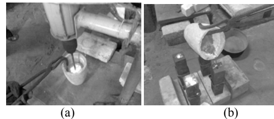
Fig 1. Preparation of SiC reinforced composites (a) Mechanical mixing of particles with ZA27 and (b) Pouring of freshly prepared composite in metal mould
